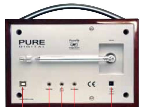
USB Connector Stereo Line Out XT-1 Speaker Output Headphone Socket Power Input
